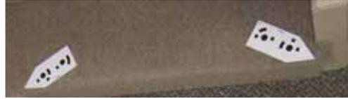
**6-** Continue up the steps and intermediate landings placing the L and R markers on the front tread edge of each appropriately numbered step. Use Landing markers to indicate opposite walls and obstructions that could interfere with chair lift operations. Landing markers should also be used on any intermediate landing as necessary to build point count to 15 targets per photo.
